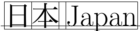
Figure 1: The width of an ordinary Japanese character, 1 zw , is set to 92.469% the design size of the Latin font, and a gap of 0.25 zw is inserted. The baseline is set to 0.12 zw above the bottom of the enclosing squares.
