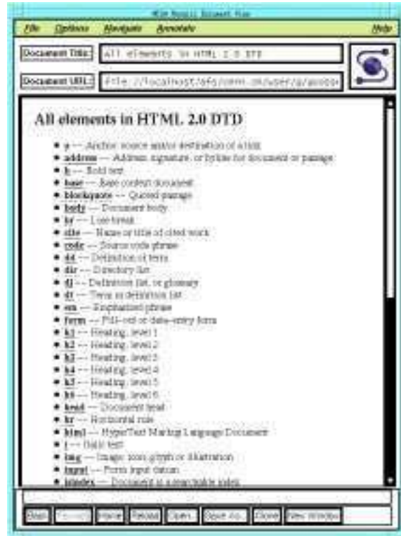
Figure 11: Hypertext description of the elements of a DTD (HTML2) as presented by the HTML browser mosaic
