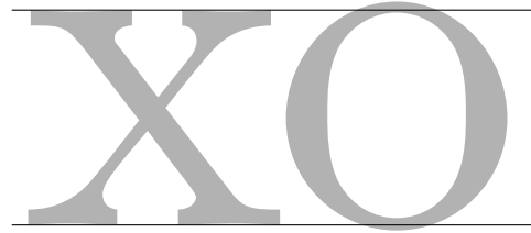
FIG. 7: The difference between the height of a glyph with a flat top segment and a glyph with a round top segment is called top overshoot . Analogously, the difference in depth is called bottom overshoot. Glyphs from the string ‘xzroesc’ are used compute the blue zone and overshoot value of the top and bottom of lowercase letters.
