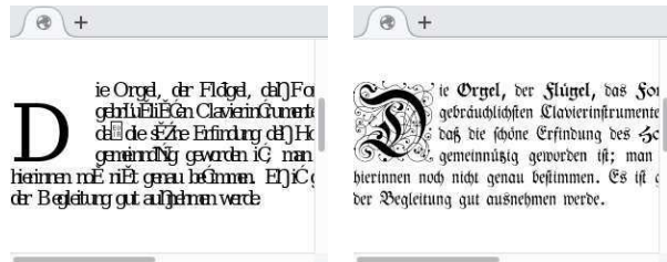
Figure 2: Screenshots of two SVG files opened in Firefox. Both were generated from the same DVI file. The left image uses font , the right path elements.
