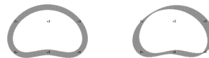
Figure 6: One path traced by two different pens [7]. The left-hand path was drawn using a circular pen, and the right-hand path used an elliptical pen inclined at 40 degrees from the x-axis.
