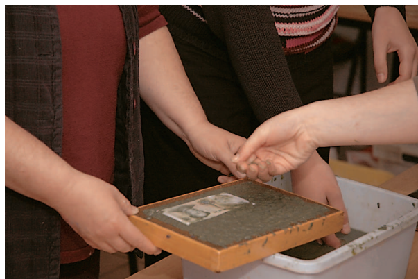
Figure 2: Helping hands: the pulp was scooped with a wire screen or sieve.
