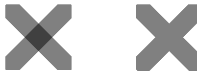
Figure 1: Two form XObjects with opacity 0.5; the right one is a group XObject.
